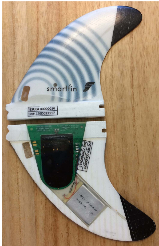
Fig. 1. The Smartfin, front and back. The top shows an unilluminated LED in the center and a small cut-out for future sensor integration. The black carbon fiber tip covers the temperature sensor. The bottom shows the PCB, rechargeable battery, and inductive charging pad.
